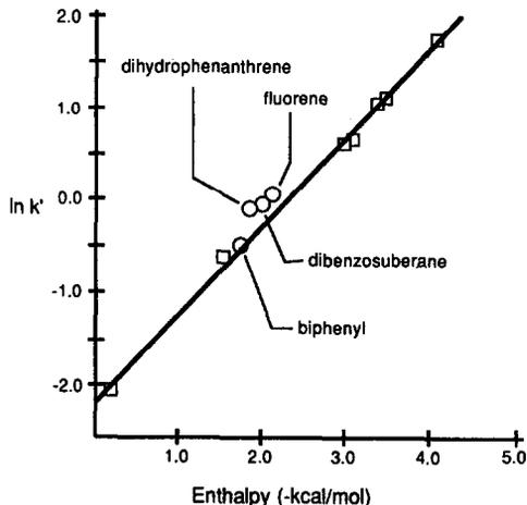
Fig. 5. Entropy-enthalpy compensation plot for (□) planar and (○) non-planar aromatic solutes on dinitrobenzoylmercapto-propylsilica (DNBMP).
