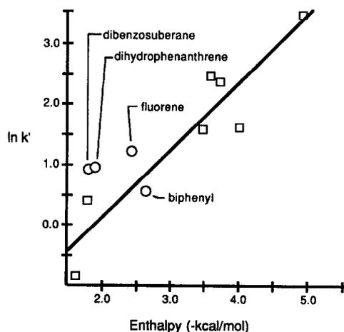
Fig. 2. Entropy-enthalpy compensation plot for (□) planar and (○) non-planar aromatic solutes on dinitroanilinopropylsilica (DNAP).
