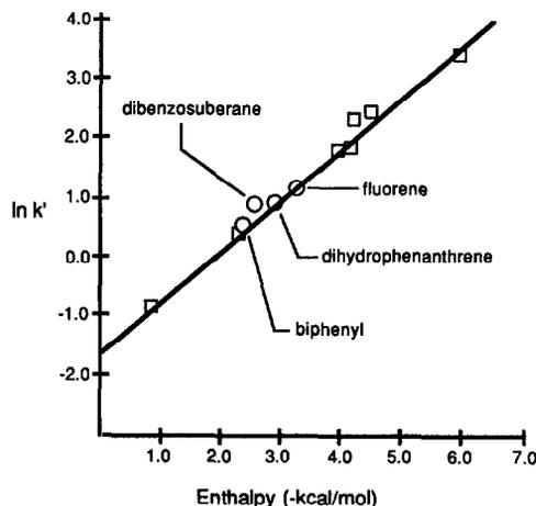
Fig. 7. Entropy-enthalpy compensation plot for (□) planar and (○) non-planar aromatic solutes on tetranitrodibenzosuberiminopropylsilica (TNDBSP).
